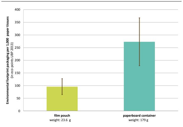
Figure 4: Environmental footprint for the packaging of 1,000 paper tissues in film pouches compared to paperboard containers (delivery distance 290 km)
